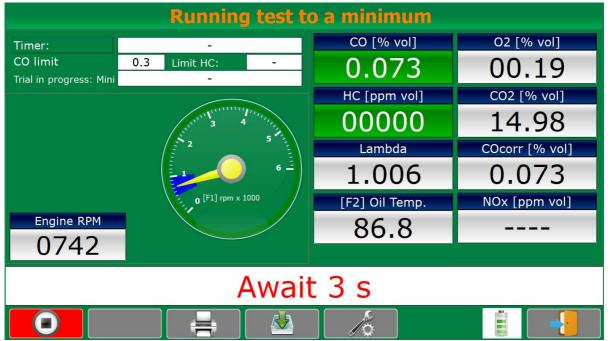
In the measure screen there are reported the measured values, the system wait for the set time for stabilization.
