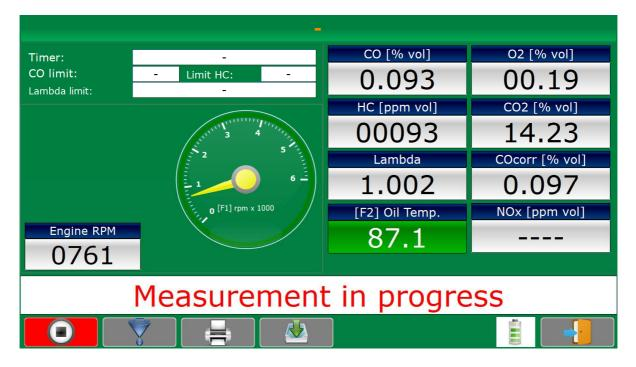
The system perform an autozero and after go in measure status. The measured values are showed in the screen.
