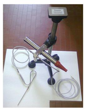
The terminal side is made with a flexible brass pipe on which the terminal must be connected. For motorbike use the rigid terminal with input from the bottom, pay attention to avoid solid parts ingress from the exhaust pipe and from the ground.
