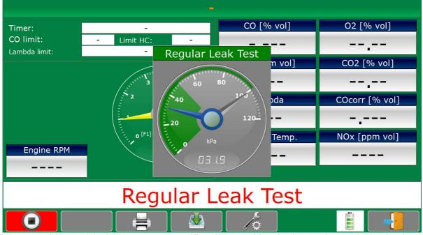
If the control is enabled, the system verifies if a positive leak test is made in the last 24 hours, if the positive test was not made, the system begin the specific procedure, in the screen are reported the operation to make and the result of the test.
