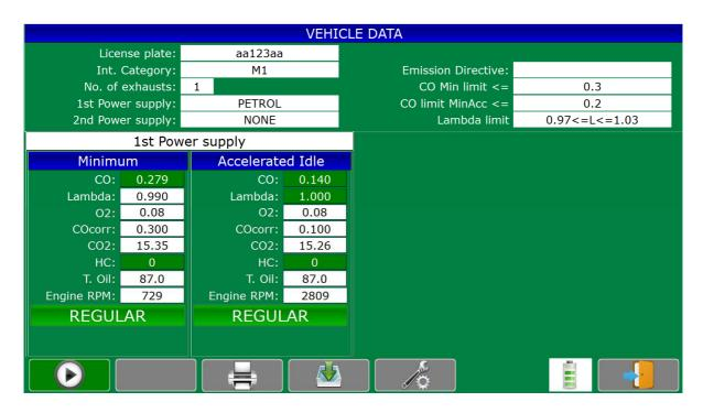
At the end, the detected values are showed in the screen with the main vehicle data, the limits applied and the result.
